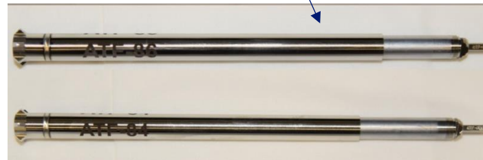
Finished Framatome microcell pellets (top) Finished rodlets containing Framatome microcell pellets before insertion in ATR (bottom)
